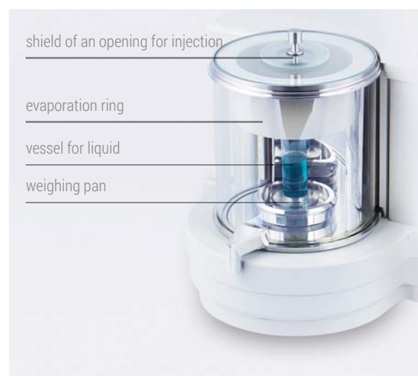
MYA 4Y.P microbalance for pipettes calibration
